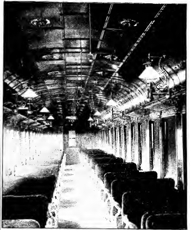
Fig. 95. INTERIOR OF FIRST-CLASS COACH. BOSTON & ALBANY RAILROAD. Turtle-Back Roof and Bracket Oil Lamps.
